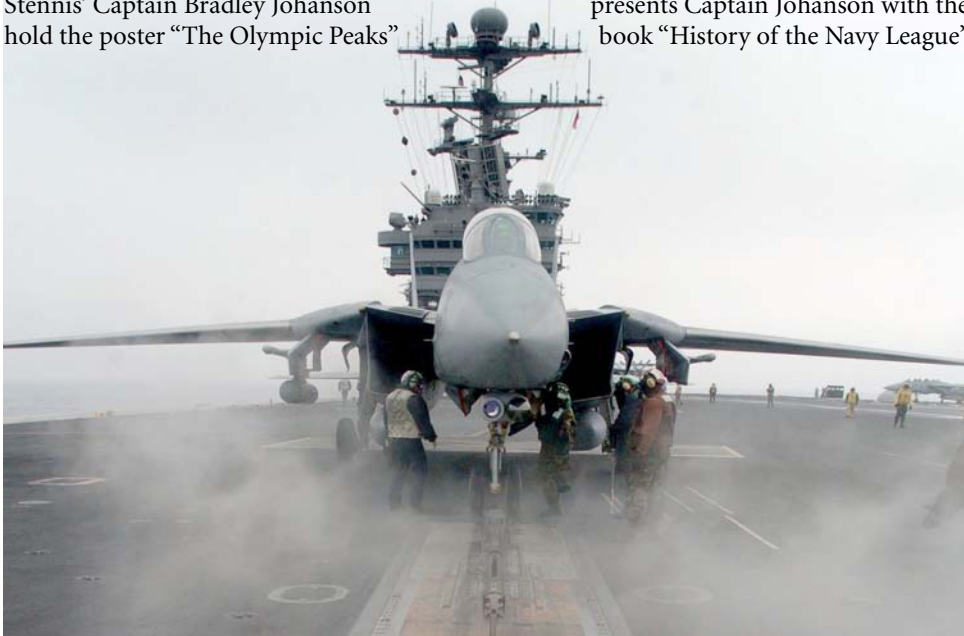
Above: An F-14D Tomcat sits poised for launch on one of four steam-powered catapults aboard the nuclear powered aircraft carrier USS John C. Stennis. Navy League members and guests toured the Stennis on December 1st as part of the League's Tours, Trips, and Adventures series.
