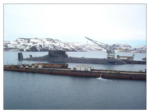
This is submarine "Typhoon" as it was called in NATO documents or "Shark" as it was called in Russia. It is considered to be the biggest submarine in the world, with over than 170 meters (515 feet) long and 23 meter (70 feet) wide. It can carry 20 ballistic nuclear missiles and there were only six of those built. Only 3 left intact, but are staying
